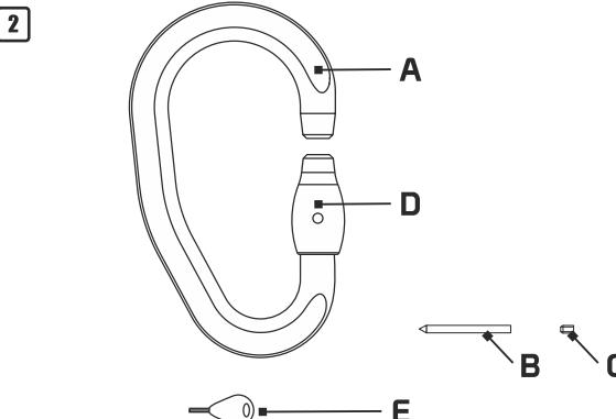
EN: (A) Stainless steel body, (B) Stainless steel bar for lanyard locking, (C) Galvanized steel grub screw, (D) Stainless steel gate, (E) Key for removal in case of emergency evacuation (not supplied).
