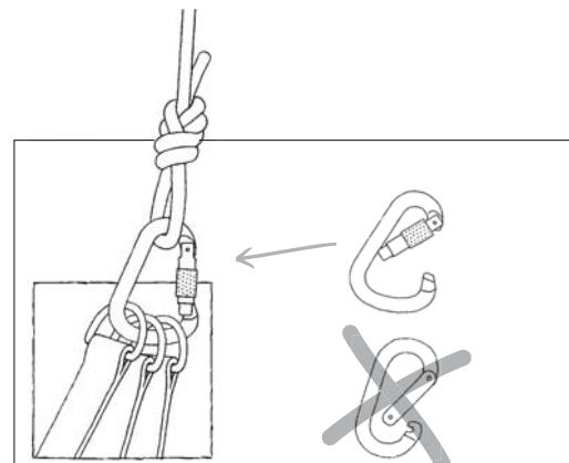
(EN) Minimum strength of fixed point 15 kN
